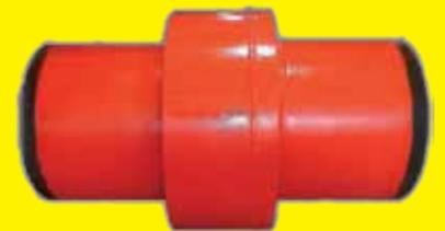
Monolithic insulation joint is a boltless structure that provides electrical resistance between the pipeline sections and adjoining structures, thus improving the effectiveness of the Cathodic Protection System.
